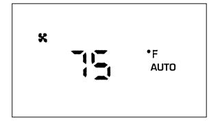
You can override the fan speed at any time. If you use the thumbwheel to override the fan speed, the EATC will continue to control the temperature but you control the fan speed. To return to auto fan control, press the AUTOMATIC button. If you are operating in one of the override functions (FLOOR, MAX A/C, etc.), automatic fan control will continue unless you rotate the fan thumbwheel. To
